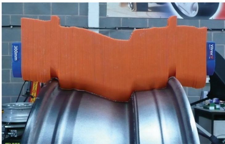
Using the gauge to profile the cross section of the wheel
